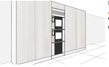
Option 1 Flush installation with XUC502 steel frame
