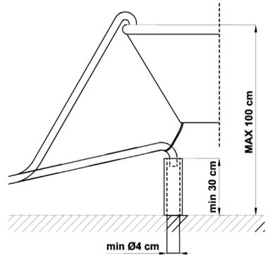
The free end should be positioned at a height of between **30 and 100 cm**, and should never be submerged in water. If a horizontal drain extension hose is used (for a maximum of 3 m) the drain hose can be placed at a maximum height of **85 cm** from the ground.
